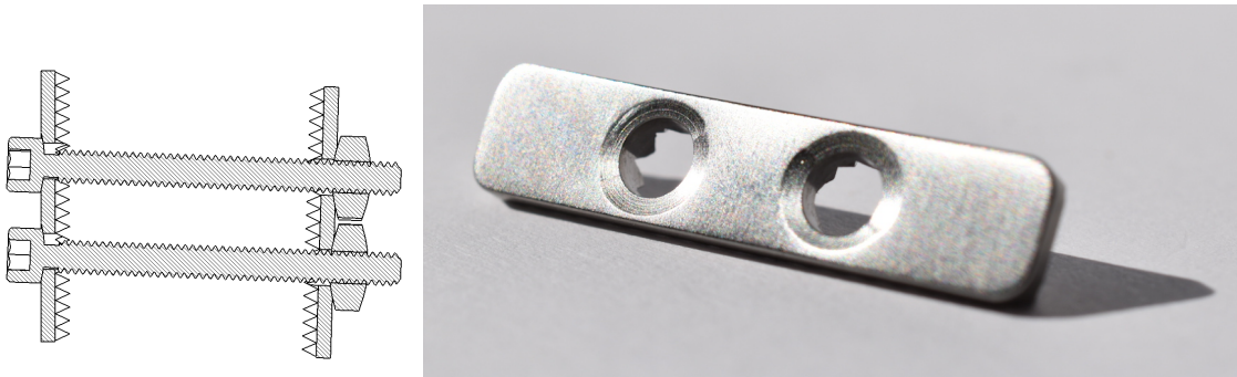
Fig. 31. Off axis loading of the aggressively teathed plates is possible through the ability of the bolts and nuts to mate with the plates. The plate has two concave mating surfaces that distribute forces when off axis loading may occur.
