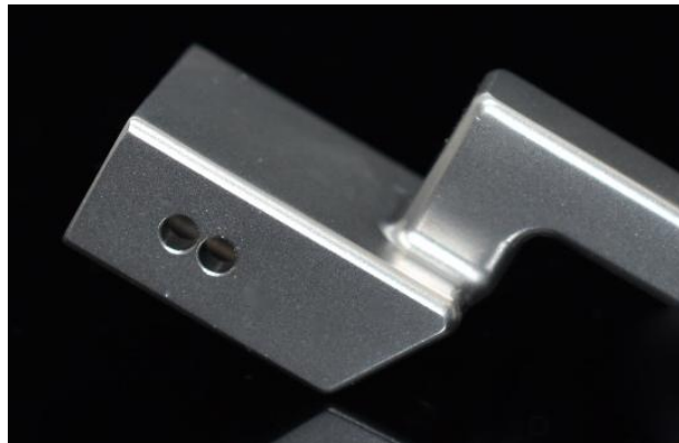
Fig.13. These two holes are used to place a parallel K-wire (KI-71-025) after the initial medial and lateral K-wires have been drilled into the respective medial and lateral epicondyle. The distance between the K-wires represents the radius of the cannulated drill bit (KTE-CLRD Drill) (Fig 12).
