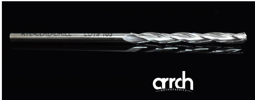
Fig. 12. A 6” length cannulated drill bit (KTE-CLRD Drill) has an outer diameter of 0.275” and an inner diameter of 0.094”, which is used to overdrill the K-wire (KI-71-025) placed parallel to the centerline of ulnohumeral rotation.
